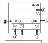
1- SET1 KEY 2:- INCREMENT KEY 3:- DECREMENT KEY 4:- DISPLAY 5:- RELAY-1 ON INDICATION 6:- RELAY-2 ON INDICATION
